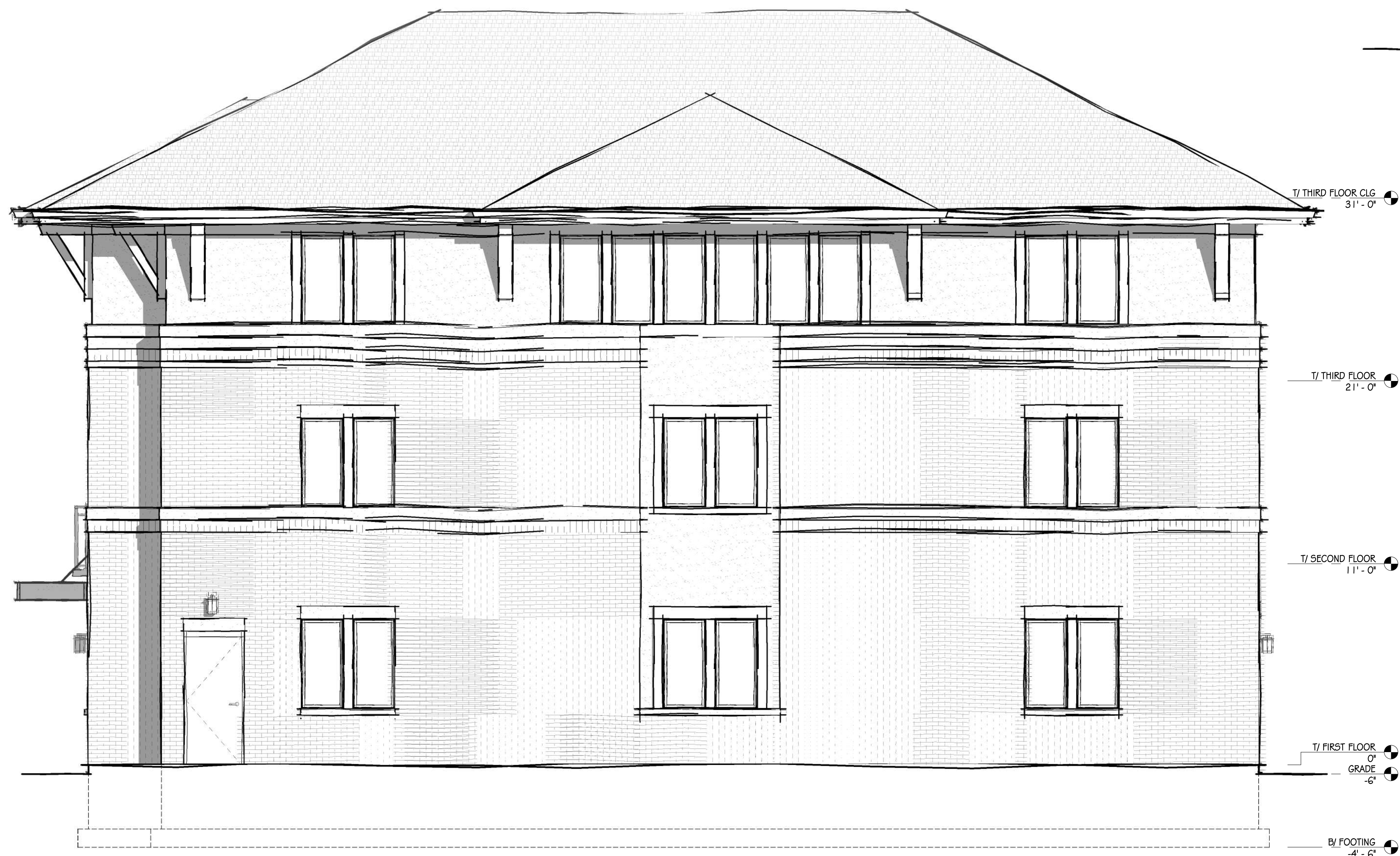
2 A-2.1 CONCEPT WEST ELEVATION SCALE: 1/4" = 1'-0"
