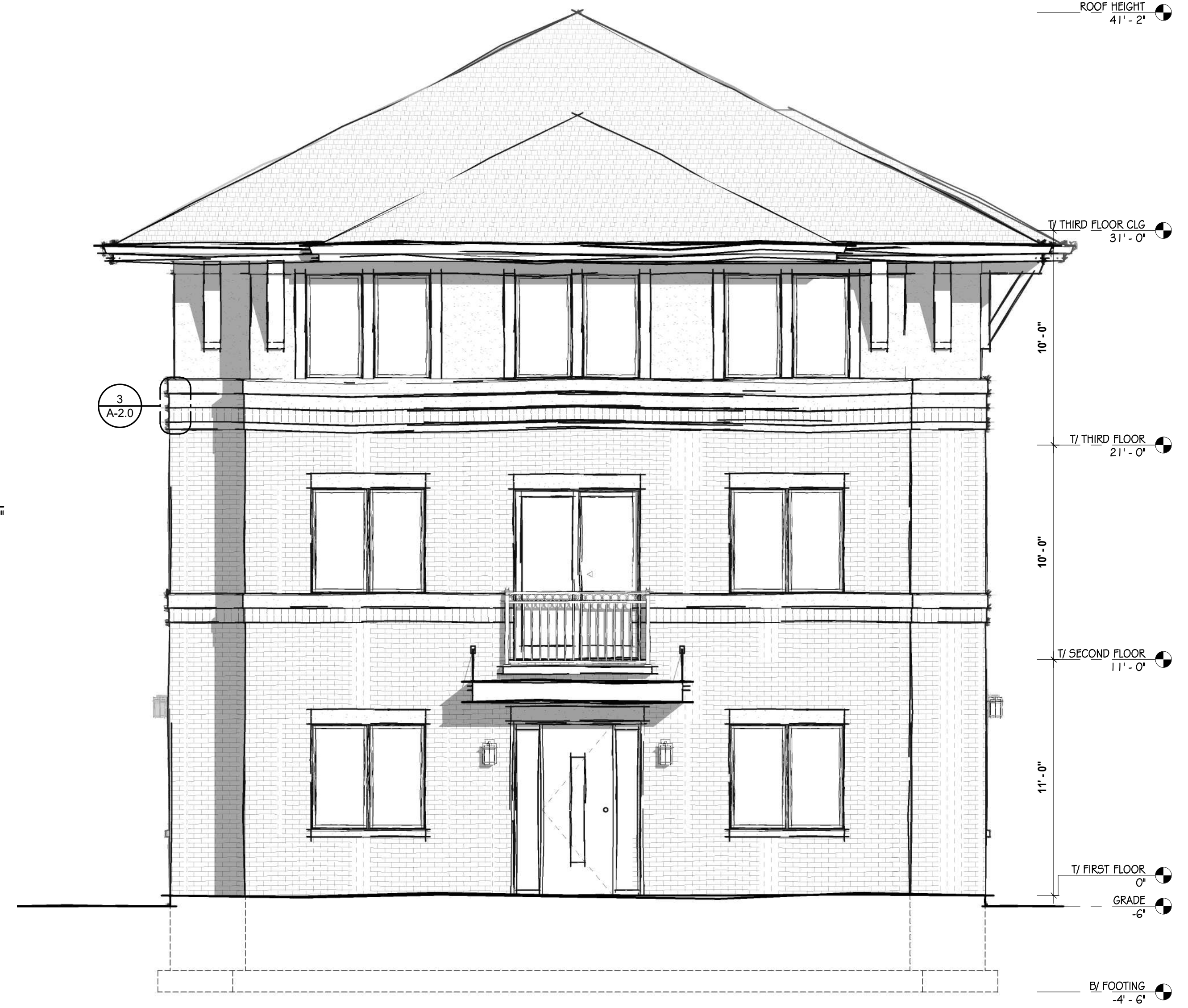
1 CONCEPT NORTH ELEVATION A-2.0 SCALE: 1/4" = 1'-0"
