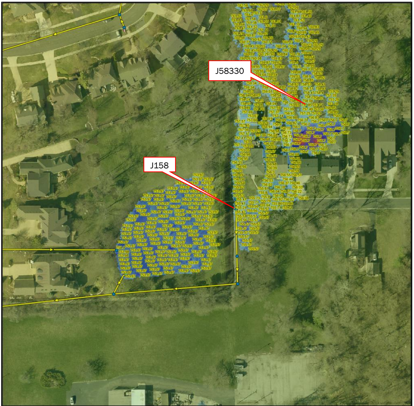
Figure 4: Existing 1-year critical duration (2-hr) inundation limits with maximum water surface spot elevations shown.
