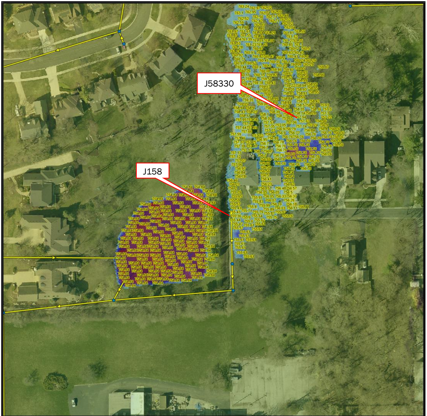
Figure 6: Existing 2-year critical duration (2-hr) inundation limits with maximum water surface spot elevations shown.
