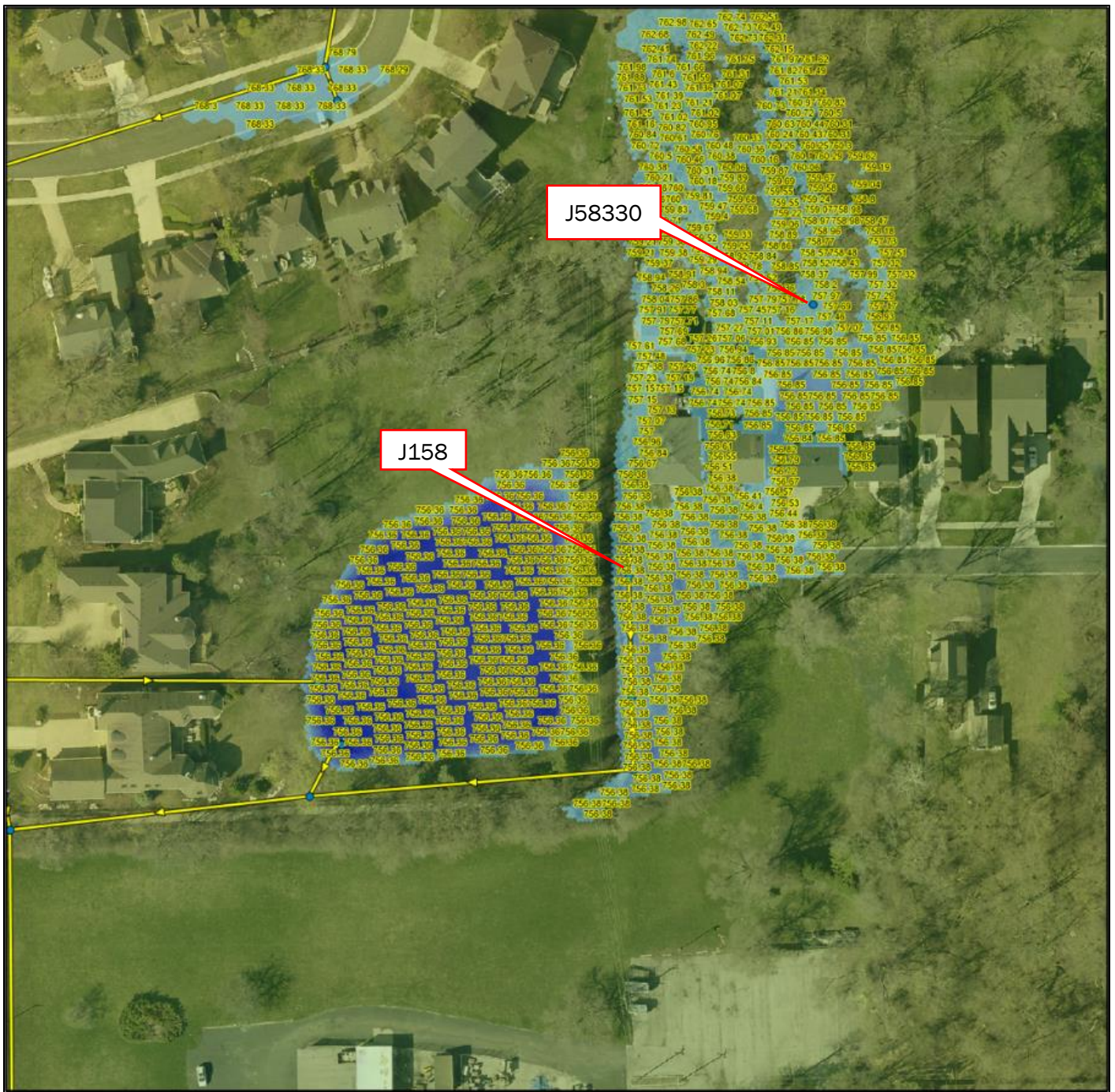
Figure 8: Existing 5-year critical duration (2-hr) inundation limits with maximum water surface spot elevations shown.
