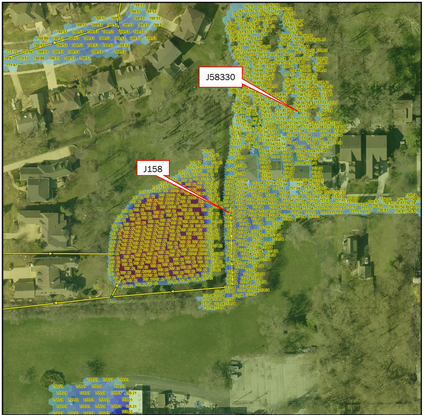
Figure 10: Existing 10-year critical duration (3-hr) inundation limits with maximum water surface spot elevations shown.
