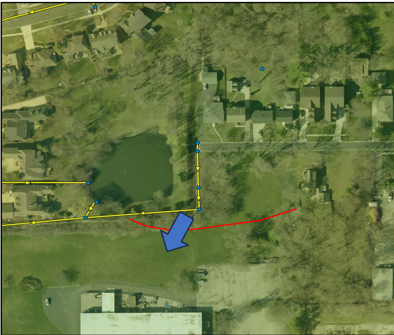
Figure 17: Location of ridgeline in red. Overtopping location shown with blue arrow.
