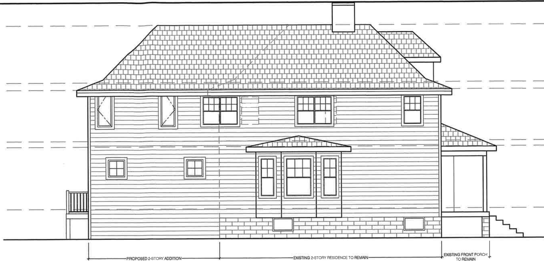
4 PROPOSED EAST ELEVATION 1/8" = 1'-0"
