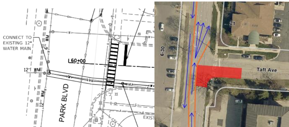
Taft & Park Blvd. 12" Water Main Connection
