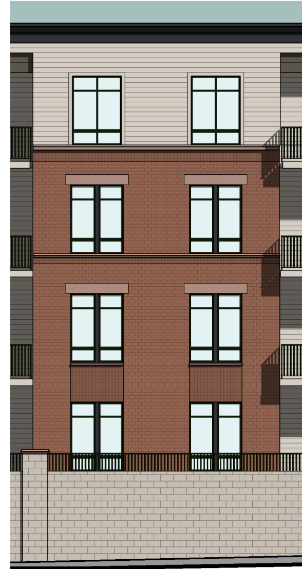
2 TYPICAL ELEVATION DETAIL SCALE: 1" = 10'-0"
