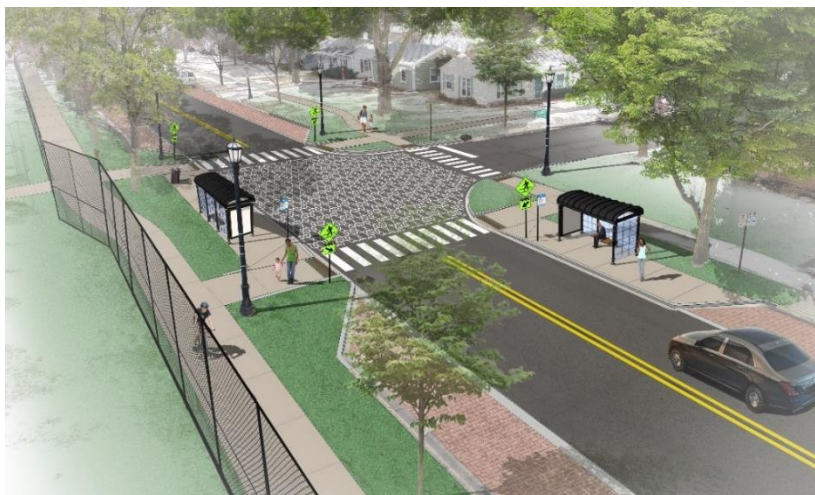
MMA used to create patterns across roadway
