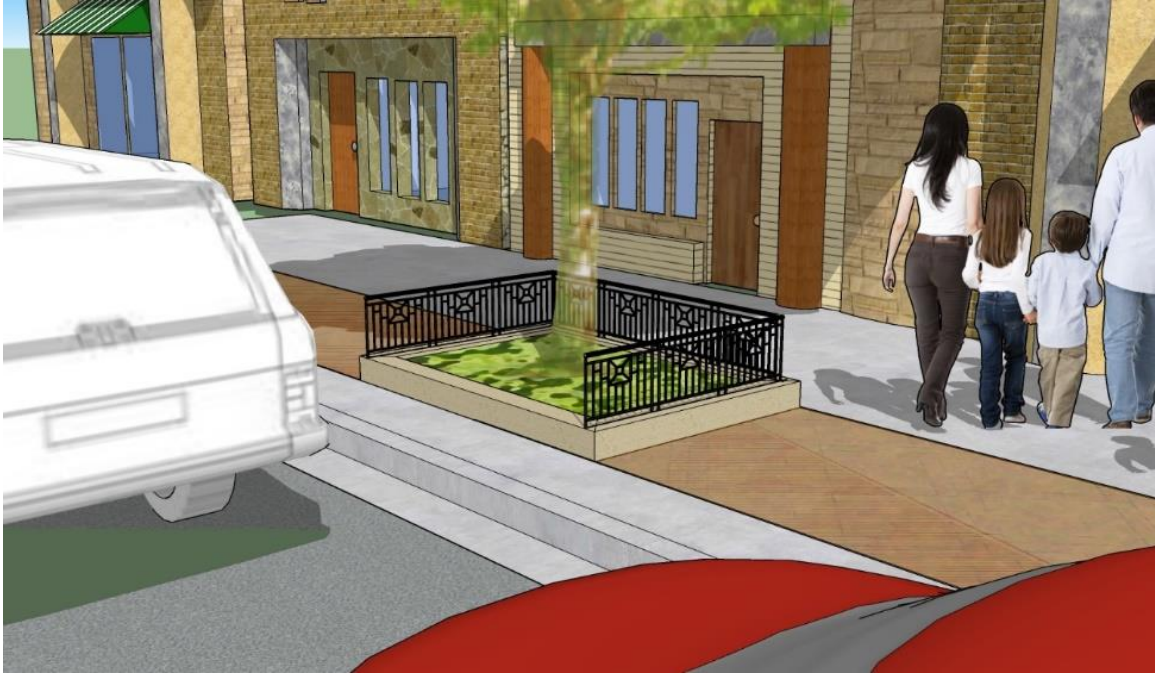
Low planter railing attached to curb
