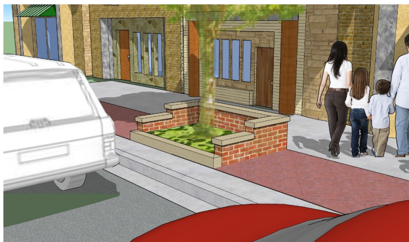
Stepped down wall on three sides
