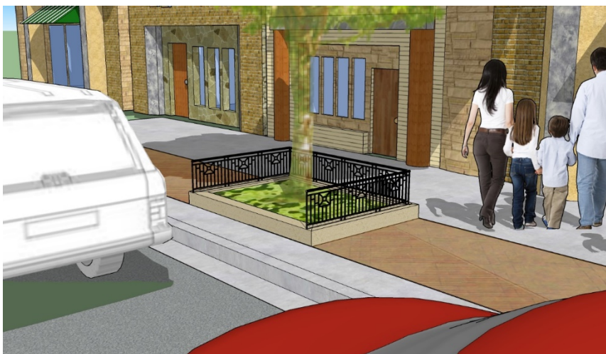
Low planter railing attached to curb
